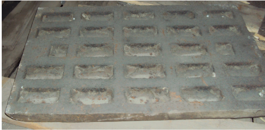
Plate 2: Cast Crusher jaw with back recesses
