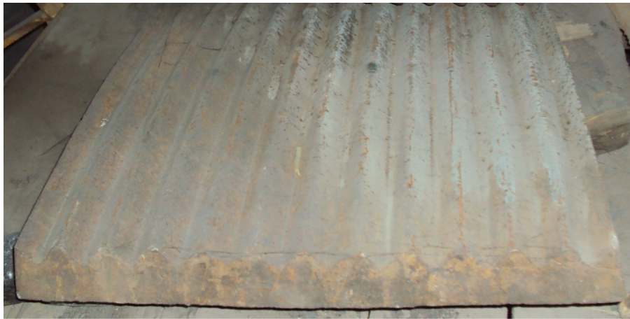
Plate 1: Cast crusher jaw with fully formed teeth
