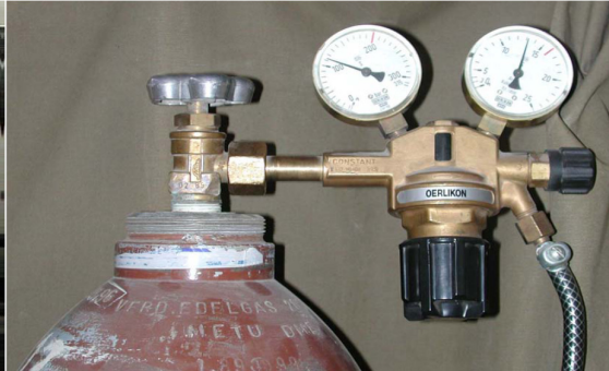
Figure 2: Shielding gas vessel and regulator
