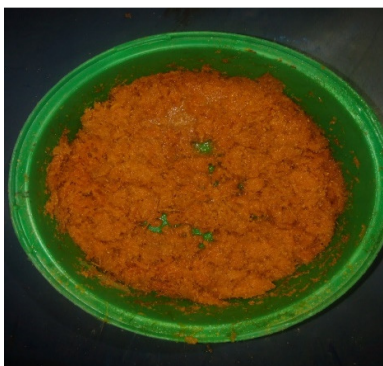
Figure 3: bamboo activated carbon impregnated with nitric acid (HNO 3 )
