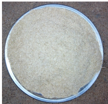
Figure 2: Crushed bamboo before impregnation
