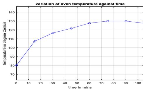
Figure 1: Variation of oven temperature against time using cake baking
