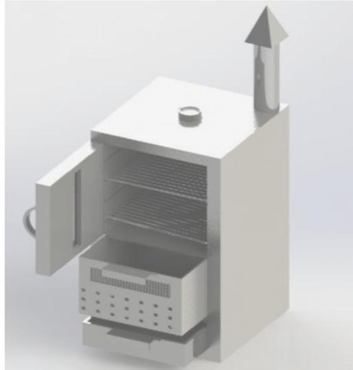
Figure 1: Fabricated biomass fired-oven
