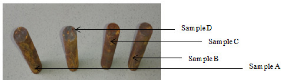
Figure 5: Samples of low carbon steel after exposure to seawater
