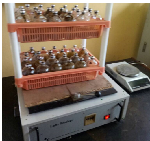
Figure 1: BMP test bottles on laboratory shaker
