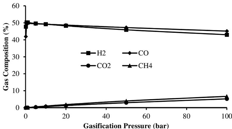
Figure 3: Effect of gasification pressure on Syngas composition (Steam to coal ratio = 0.5, Oxygen to coal = 0.2, Gasification Temperature = 1100 °C)
