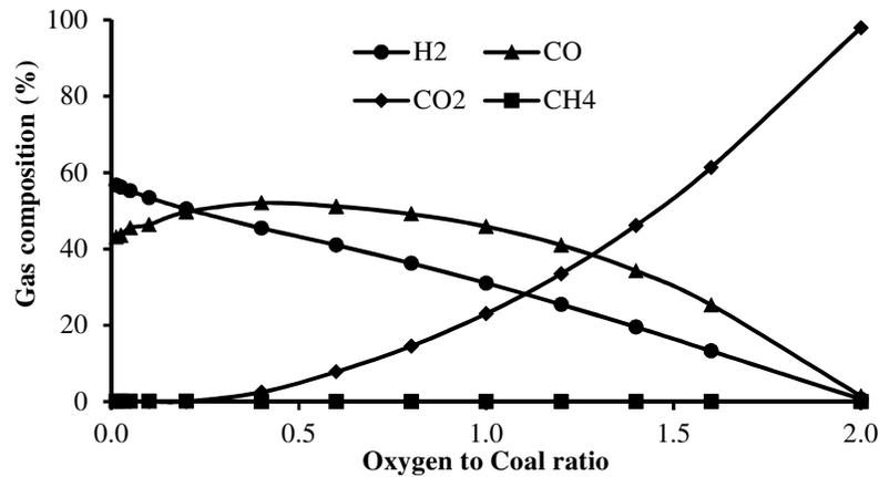
Figure 4: Effect of oxygen to coal ratio on syngas composition (Steam to coal ratio = 0.5, Gasification temperature = 1100 °C, Gasification pressure = 1bar)
