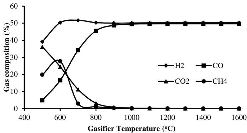
Figure 2: Effect of gasification temperature on syngas composition (Steam to Coal ratio = 0.5, Oxygen to Coal = 0.2, Gasification pressure = 1bar)
