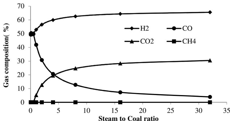
Figure 5: Effect of Steam to Coal ratio on Syngas composition (Oxygen to coal = 0.2, Gasification Temperature = 1100 °C, Gasification pressure = 1bar)
