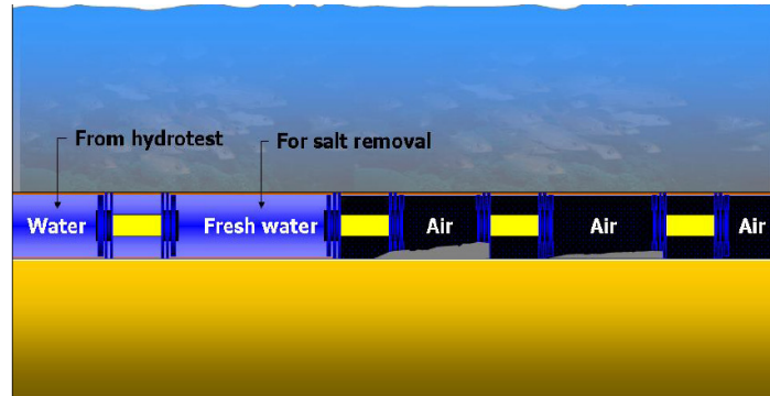
Figure 4: Gas pipeline dewatering (Russell, 2005)
