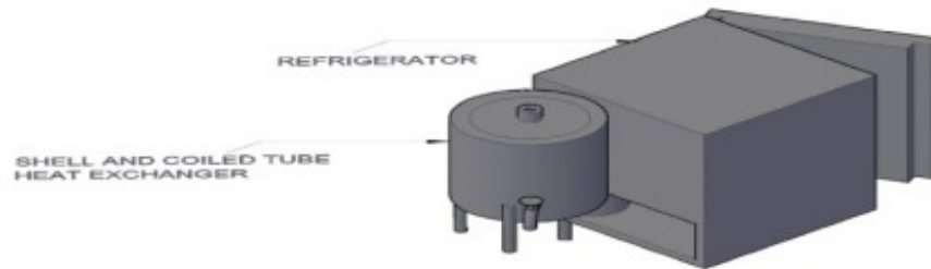
Figure 3: Assembly drawing of fitted shell and coiled tube heat exchanger to the refrigerator
