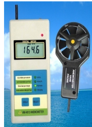
Figure 2: Am-4201 Vane probe digital anemometer (Musa et al., 2018)
