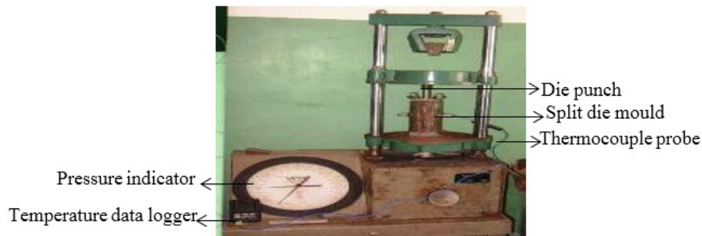
Figure 1: Experimental setup of squeeze casting process
