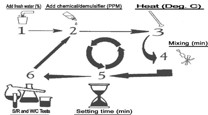
Figure 1: Simplified experimental procedure for crude oil desalting process (Al-Otaibi *et al.*, 2003)
