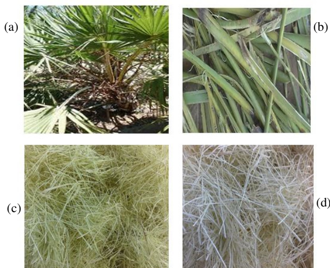
Figure 2: Images of (a) Hyphaene thebaica plant (b) Hyphaene thebaica stalk (c) raw pulverized Hyphaene thebaica fiber (d) Mercerized Hyphaene thebaica fiber
