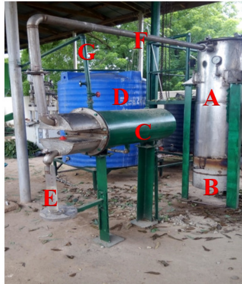
Plate 1: Steam distillation pilot plant for extracting essential oil from lemon grass
