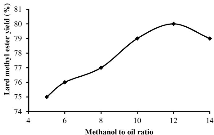
Figure 1: Effect of methanol to oil ratio on lard methyl ester yield
