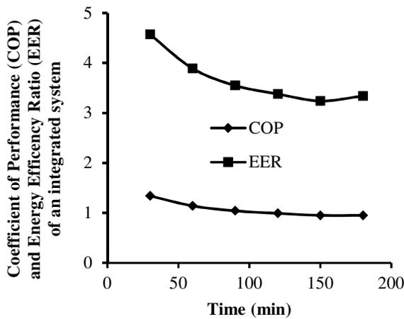
Figure 11: Comparison of COP and EER of air conditioning system at different times
