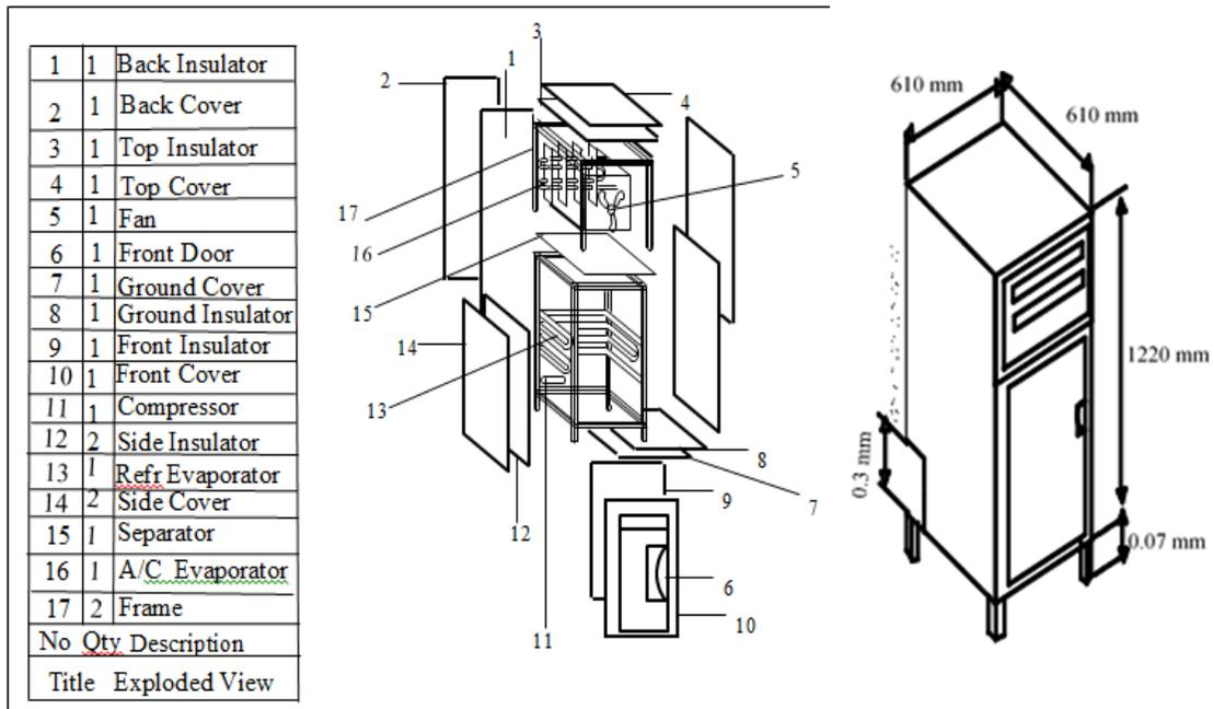
Figure 9: Exploded view of the integrated cooling system
