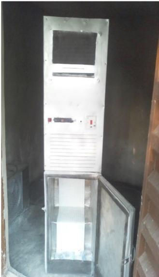
Plate 1: The developed single unit air-conditioning and refrigerating system
