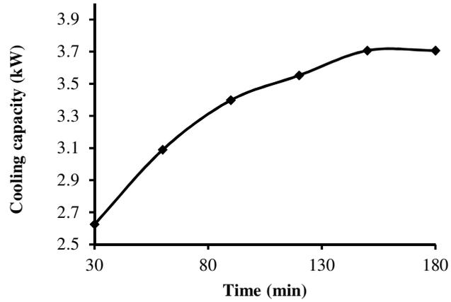
Figure 10: Cooling capacity of air conditioning system at different times
