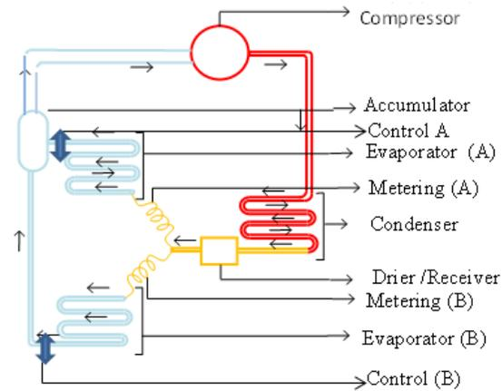
Figure 1: Plant-flow diagram for the integrated cooling system
