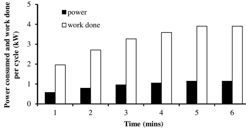
Figure 13: Comparison of the power consumed and work done per cycle
