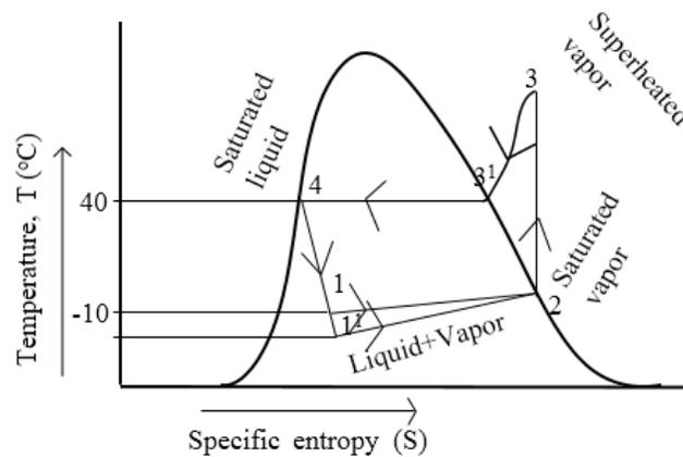
Figure 2: Temperature-entropy (t-s) diagram for integrated cooling system
