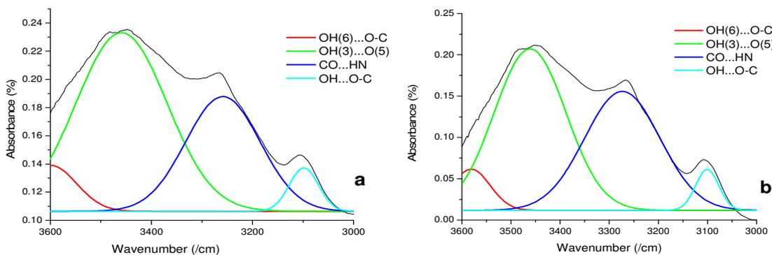
Figure 6: FTIR spectra of (a) prawn chitin and (b) shrimp chitin between  $3600 - 3000\text{ cm}^{-1}$  showing inter and intra molecular hydrogen bond positions
