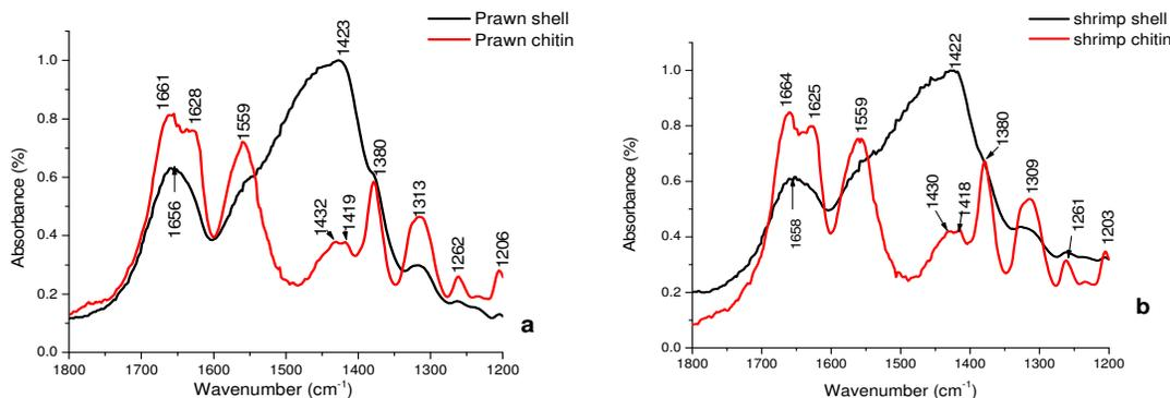
Figure 5: FTIR spectra of (a) prawn shell and prawn chitin (b) shrimp shell and shrimp chitin between  $1800 - 1200\text{ cm}^{-1}$
