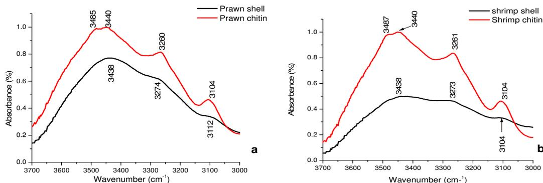
Figure 4: FTIR spectra of (a) prawn shell and prawn chitin (b) shrimp shell and shrimp chitin between  $3700\text{--}3000\text{ cm}^{-1}$
