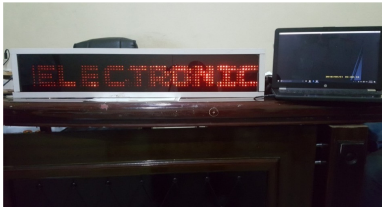
Figure 7: Completed work displaying information and connected to computer showing video
