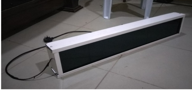
Figure 6: Pictorial view of complete case of unit (88 cm × 17.7 cm × 8 cm)
