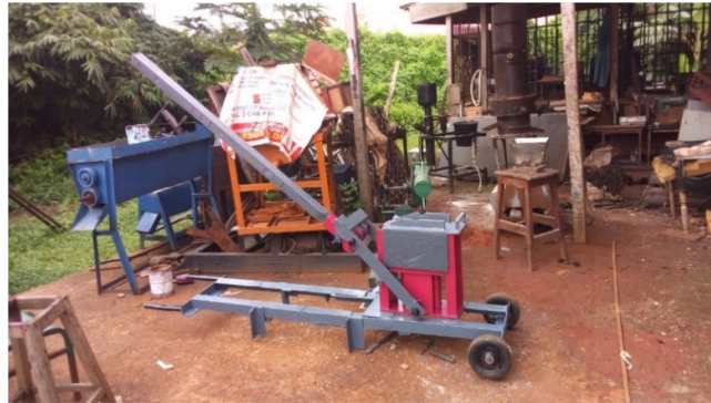
Figure 8: Finished stabilized compressed earth brick moulding machine
