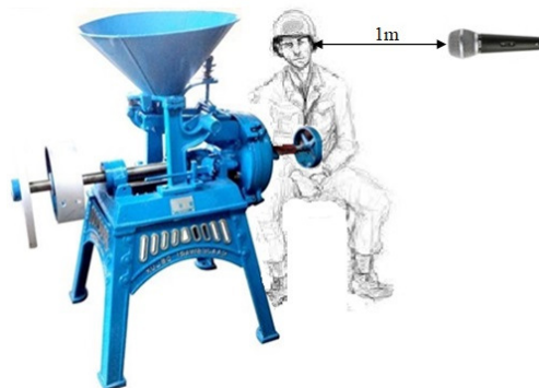
Figure 5: Microphone placements for measuring noise spectrum at grinding machines operators head level
