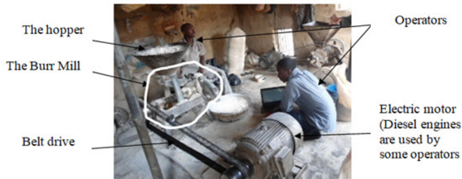
Figure 2: The burr milling machine meant for heavy duty works
