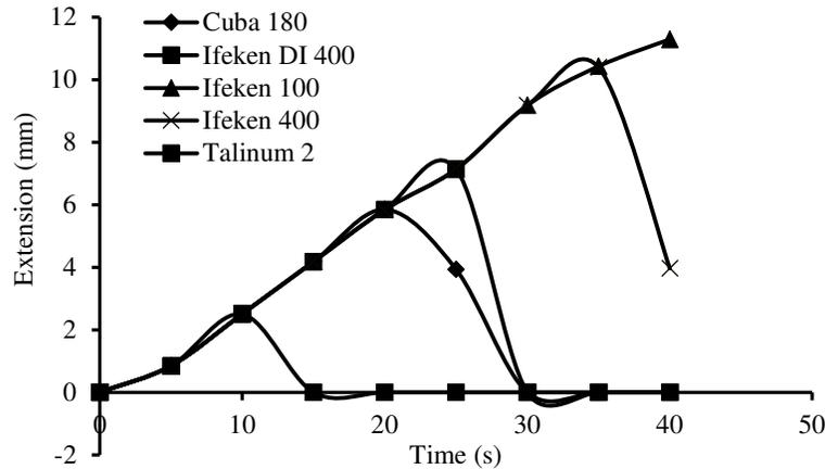
Figure 4: Comparison of extension at different times for the various fibre species
