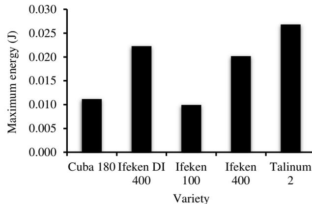
Figure 5: Maximum energy exerted on the fibres before rupture
