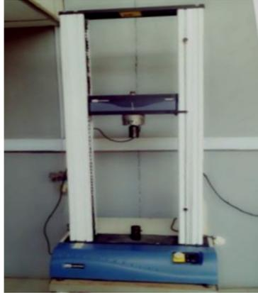
Plate 1: Universal Instron testing machine
