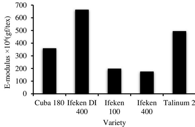
Figure 6: Modulus of elasticity for the various kenaf species
