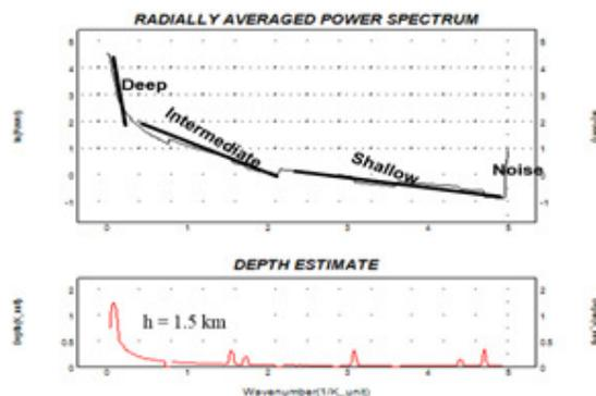
Figure 4: Radial spectrum and depth estimate plots from the aeromagnetic data
