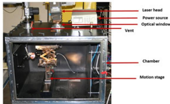
Figure 1: Experimental set-up used for the small and large beam diameters
