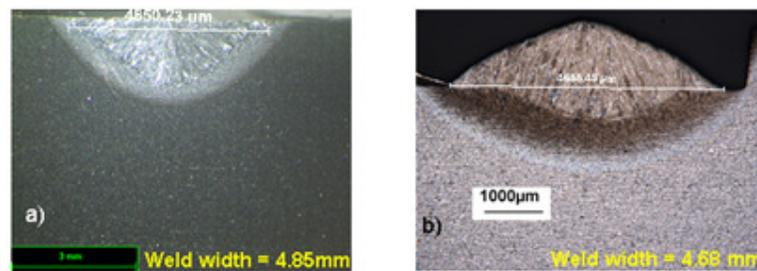
Figure 6: Comparison of weld width with build width produced with energy density of 6.7 kJ/cm<sup>2</sup> (28 kW/cm<sup>2</sup> and 240 ms) and beam diameter of 5.00 mm a) solid melting and b) powder melting
