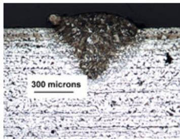
Figure 12: Deposited tracks for 0.2 mm powder layer thickness, power density of  $5350 \text{ kW/cm}^2$  and interaction time of 2 ms with keyhole characteristic
