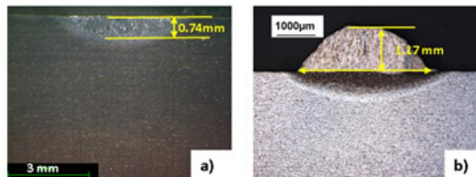
Figure 3: Comparison of the depth of penetration with build height at a constant energy density of 34 J/mm<sup>2</sup> (28 kW/cm<sup>2</sup> and 120 ms) and beam diameter of 5.00 mm for a) solid melting and b) powder melting
