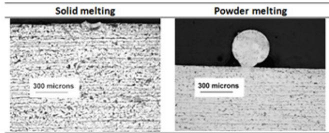
Figure 8a: Comparison of bead-on-plate weld with a single layer powder deposition at constant power density of  $640 \text{ kW/cm}^2$ , interaction time of 10 ms and layer thickness of 0.2 mm
