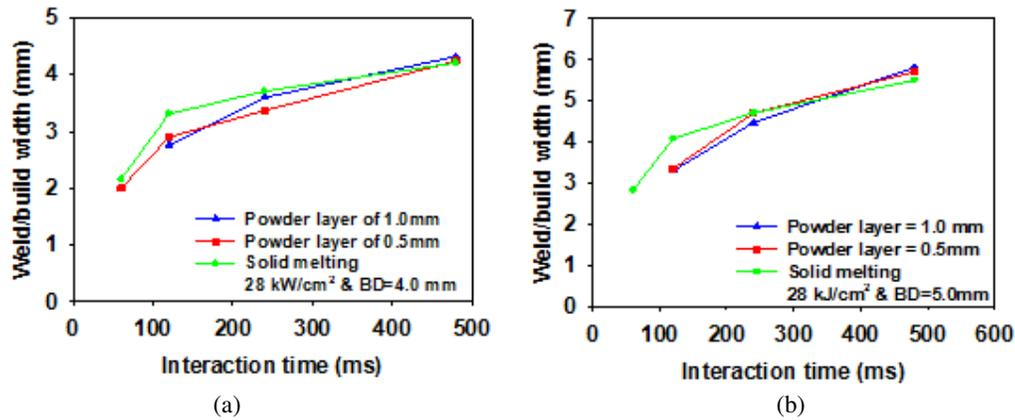
Figure 7: Comparison of the weld width with build width for the same energy density and layer thickness for beam diameters of (a) 4.0 mm and (b) 5.0 mm (Note: green lines are penetration in solid melting)
