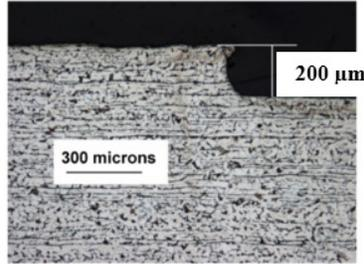
Figure 2: A groove of 0.20 mm used for powder melting with a bead diameter of 0.10 mm
