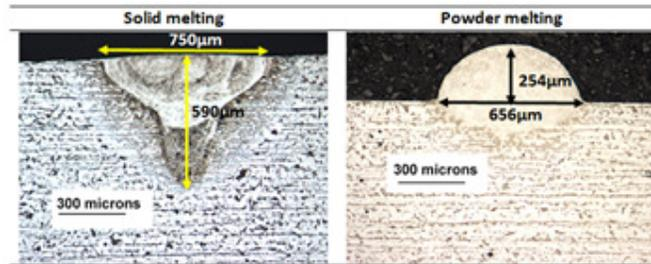
Figure 11a: Comparison of bead on plate weld with a single layer powder deposition at constant power density of 5350 kW/cm<sup>2</sup>, interaction time of 2 ms and layer thickness of 0.2 mm
