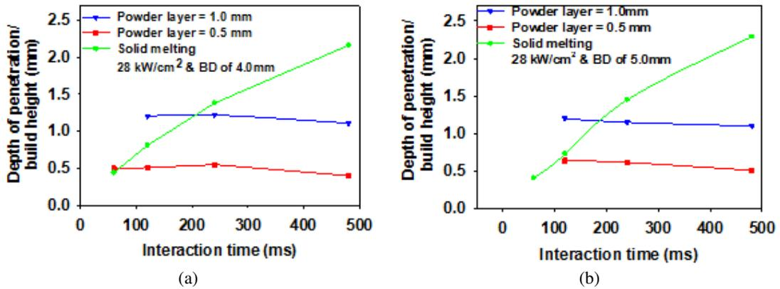
Figure 4: Comparison of the depth of penetration with build height for the same energy density and layer thickness for beam diameters of (a) 4.0 mm and (b) 5.0 mm (Note: green lines are penetration in solid melting)
