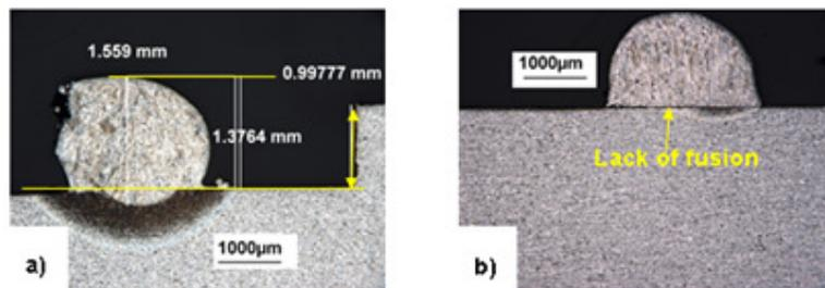
Figure 5: Examples of defects in powder melting a) humping formation b) lack of fusion below minimum energy for fusion
