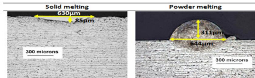
Figure 9: Comparison of bead on plate weld with a single layer powder deposition at constant power density of  $2670 \text{ kW/cm}^2$ , interaction time of 4 ms and layer thickness of 0.2 mm
