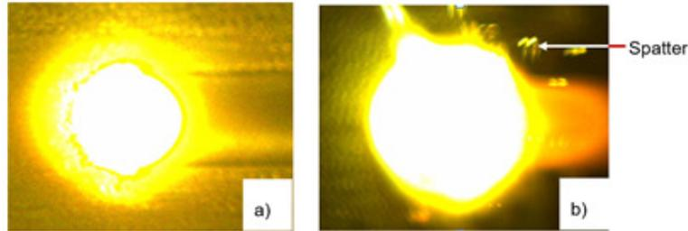
Figure 13: Melting characteristics in two different materials for the same processing conditions (a) solid melting (b) powder melting
