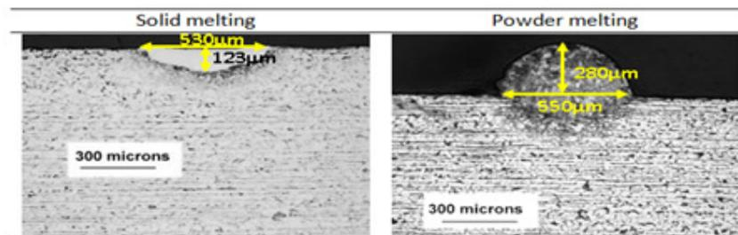
Figure 10a: Comparison of bead on plate weld with a single layer powder deposition at constant power density of  $2670 \text{ kW/cm}^2$ , interaction time of 8 ms and layer thickness of 0.2 mm
