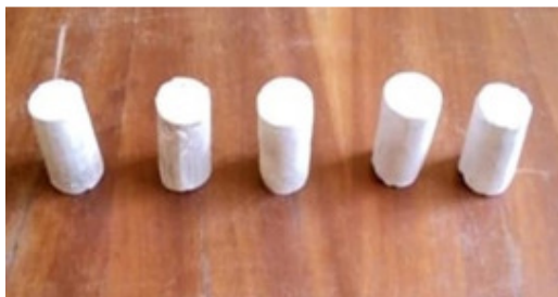
Figure 1: Cordierite samples numbered A to E sintered at 1200 °C for 2 hours
