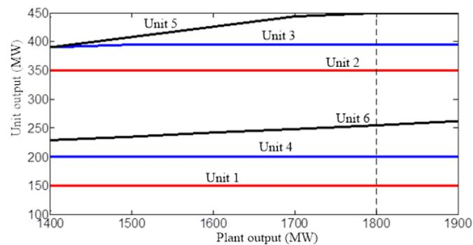
Figure 3: Output of each generating unit versus the total plant output
