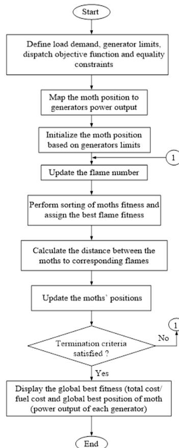
Figure 1: Moth flame optimization algorithm flow chart
