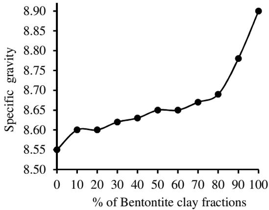
Figure 1: Variation of specific gravity with clay fraction for Bentonite-Koko clays
