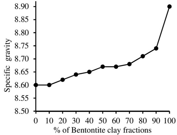
Figure 2: Variation of specific gravity with clay fraction for Bentonite-Ubeji clays
