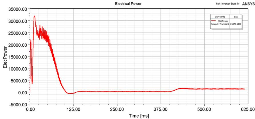
Figure 15: Six-phase inverter-start IM electrical power plot
