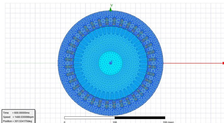
Figure 2: FEA Mesh plot of the six-phase inverter-start IM
