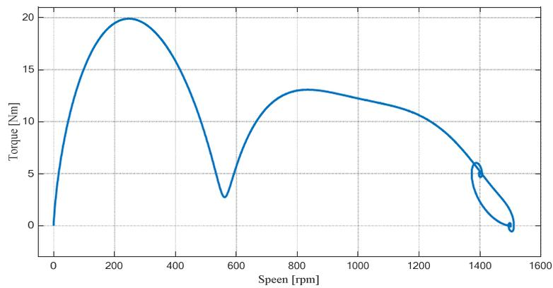
Figure 13: Six-phase inverter-start IM torque-speed characteristic in d-q variables
