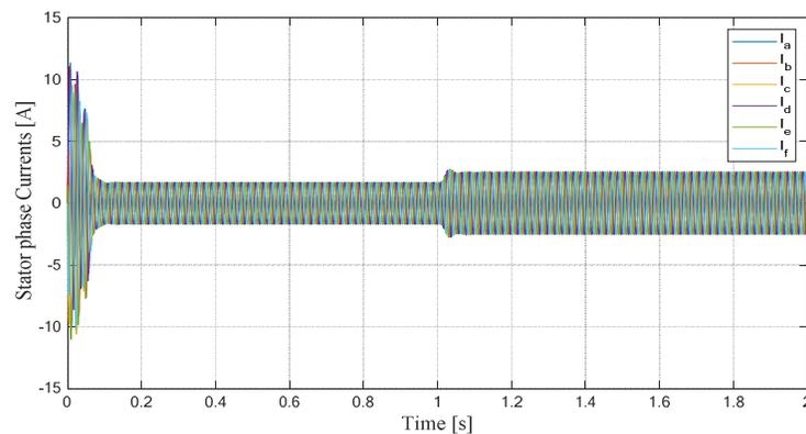
Figure 11: Six-phase inverter-start IM stator phase currents in d-q variables
