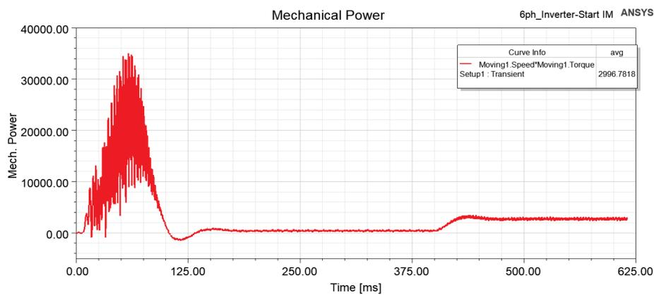
Figure 16: Six-phase inverter-start IM mechanical power plot
