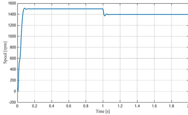
Figure 7: Six-phase inverter-start IM speed characteristic in d-q variables
