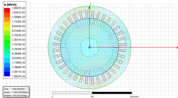
Figure 17: Six-phase inverter-start IM magnetic flux lines showing the magnetic vector potential
