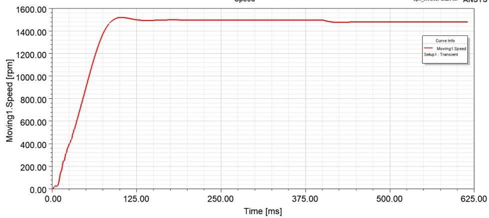
Figure 8: FEA Six-phase inverter-start IM speed characteristic
