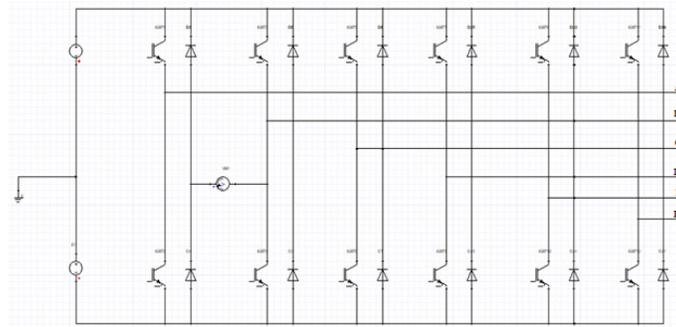
Figure 4: Six-phase voltage source inverter circuit
