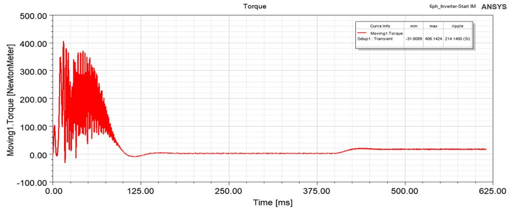
Figure 10: FEA Six-phase inverter-start IM torque characteristic
