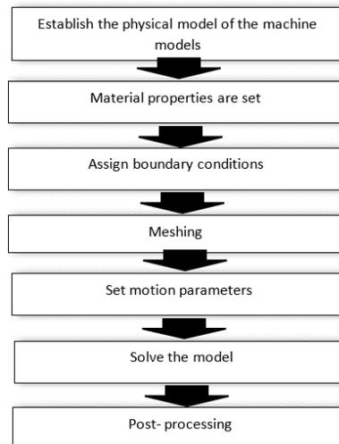
Figure 5: ANSYS FEA software modelling procedure
