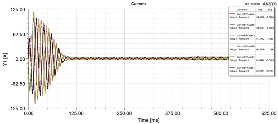
Figure 12: FEA Six-phase inverter-start IM stator phase currents
