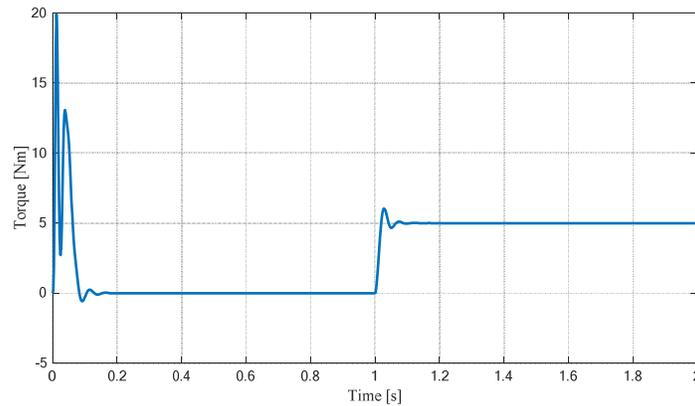
Figure 9: Six-phase inverter-start IM torque characteristic in d-q variables
