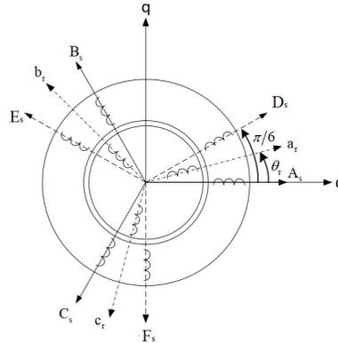
Figure 1: Six-phase induction motor stator and rotor phasors
