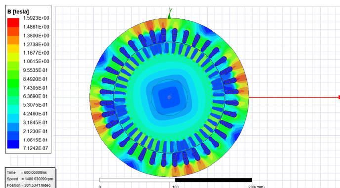
Figure 18: Six-phase inverter-start IM magnetic flux density magnitude
