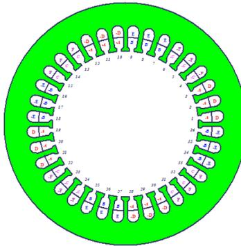
Figure 3: Winding-clock diagram of the six-phase induction motor stator
