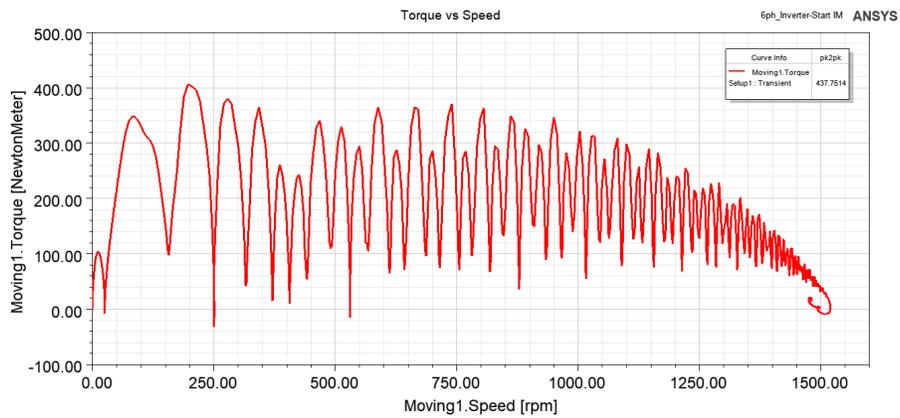
Figure 14: Six-phase inverter-start IM torque-speed characteristic
