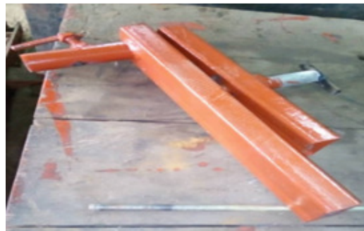
Figure 6: Carriage mechanism during construction
