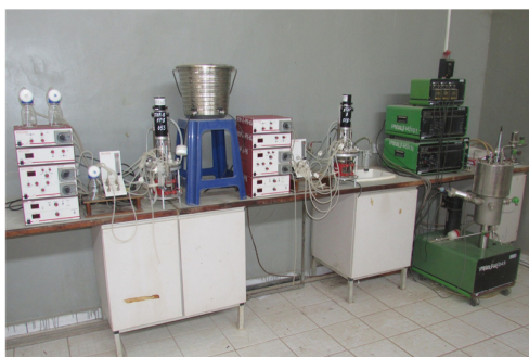
Plate 1: Laboratory reactors with automatic pH and temperature controls
