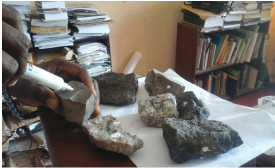
Plate I: Filling the gravels drilled holes with thermal grease
