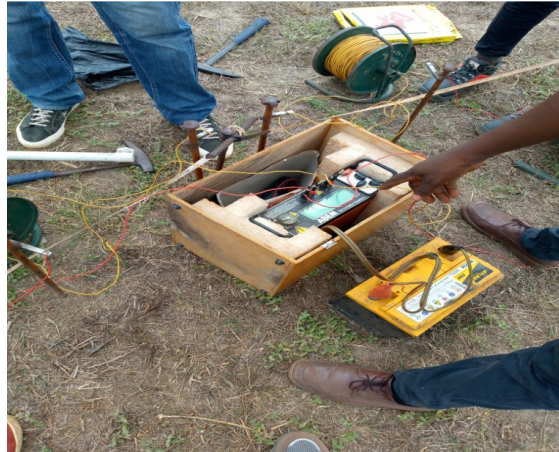
Plate 1: ABEM SAS 1000B Model Terrameter and electrode configuration during data acquisition
