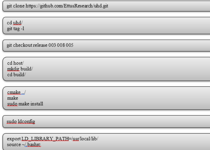
Figure 1: Building the UHD for the USRP B210 SDR (Behan et al., 2017; Aggrawal and Vachhani, 2017)
