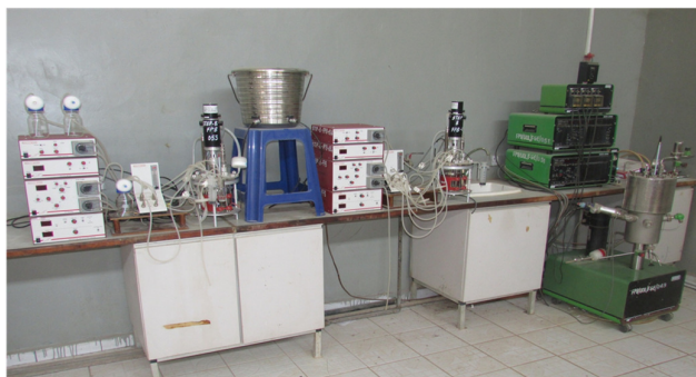
Plate 3: Laboratory reactors with automatic pH and temperature controls
