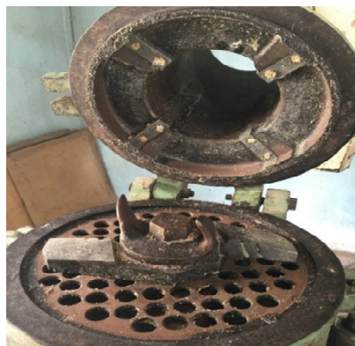
Plate 2: Inner structure of JEFCO crusher
