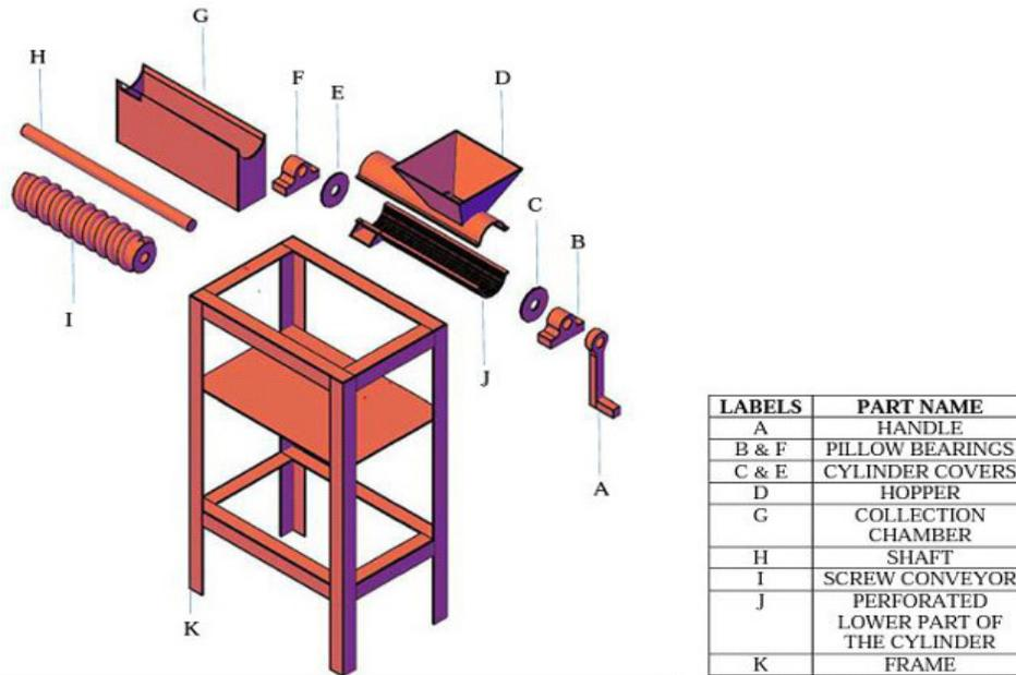
Figure 1: 3D computer aided design model of the modified juice extractor
