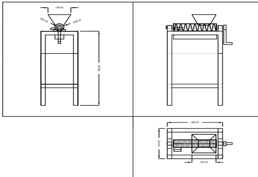
Figure 2: Orthographic view of the modified juice extractor
