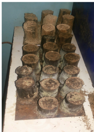
Figure 2: Briquettes (wet) immediately after extrusion from machine
