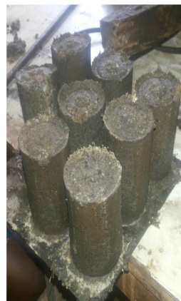
Figure 3: Briquettes (dried at temperature 28 °C) after ten days
