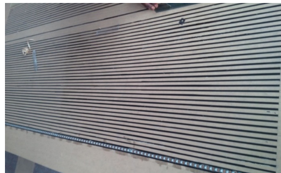
Figure 4: Cutting out of the Black PCB
