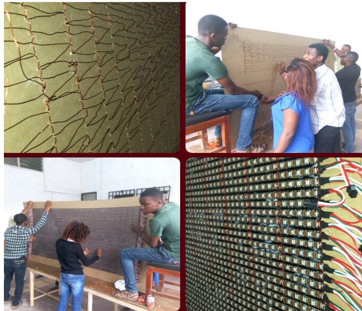
Figure 7: Transformer copper wires were passed through the holes in patterns in order to effectively hold the strips to the board
