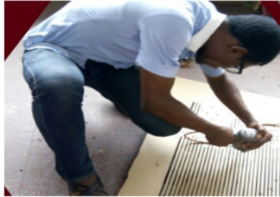
Figure 6: Drilling the pilot holes
