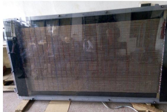
Figure 11: Mounting of the casing onto the graphics display
