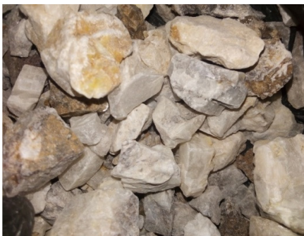
Figure 1: The picture of the barite ore from Dadin Kowa in Gombe State
