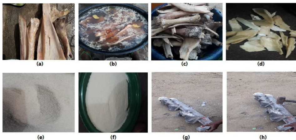
Figure 1: (a) As received cow bones (b) soaking of cow bones in detergent water (c) sun dried cow bones (d) crushed cow bones (e) ground cow bone particulates (f) sieved (150 to 300 \mu\text{m} ) cow bone particulates (g) aluminium scrap (h) re-sizing (cutting) of the scrap
