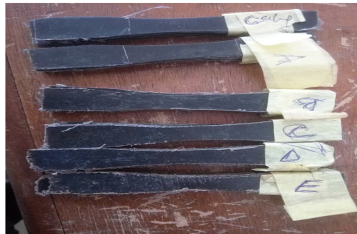
Plate VII: Dumbbell specimen for tensile strength test ASTM D-638
