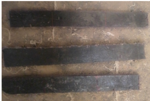
Plate IX: Flexural strength test specimen ASTM D-790
