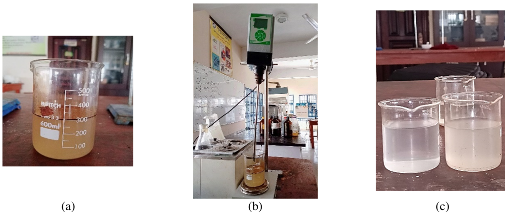
Figure 2: Coagulation jar test experimental procedure describing (a) 300 ml of the raw water transferred to a beaker (b) stirring the mixture of the coagulant and the water sample using a mechanical stirrer (c) clarified water sample
