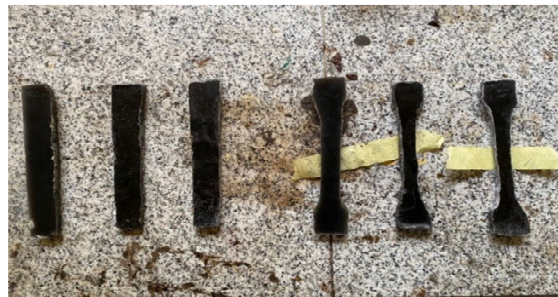
Figure 1: Tensile and flexural test samples (the first three samples at the right were prepared for tensile testing while the first three on the left were prepared for flexural testing)
