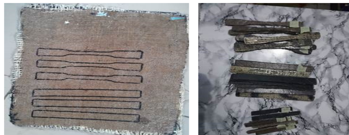
Figure 5: Mechanical samples before and after being cut according to ASTM
