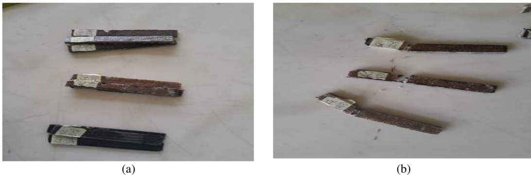
Figure 9: Impact test specimen before testing (a) and after testing (b)
