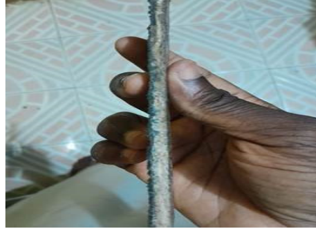
Figure 6: 5 mm thickness of one of the laminates produced
