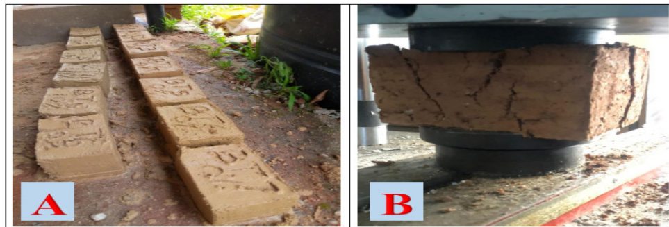
Figure 2: (a) Casted earth block samples (b) Earth block samples during crushing
