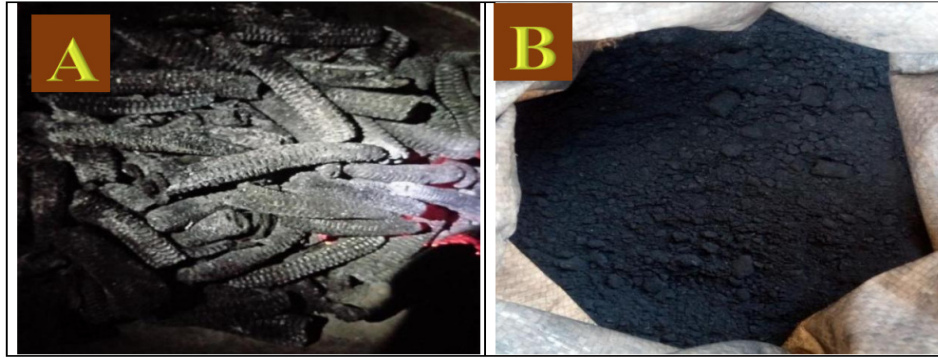
Figure 1: (a) Corncoobs during incineration (b) Corncoobs ash after incineration.
