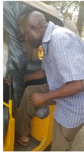
Figure 8: A passenger in bending posture while entering the tricycle due to limited clearance height
