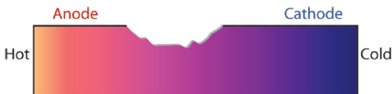
Figure 15: Thermogalvanic corrosion process (Anaee and Abdulmajeed, 2016)
