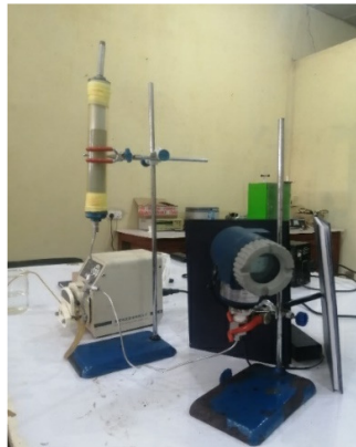
Figure 3: Core flooding (imbibition) set up
