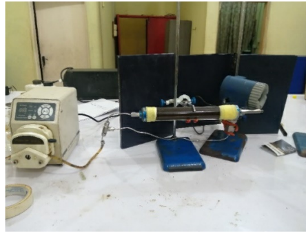
Figure 4: Core flooding (drainage process) set up
