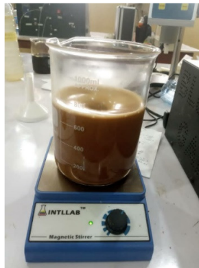
Figure Error! No text of specified style in document.: Preparation of polymer slug for both Guar Gum and Gum Arabic
