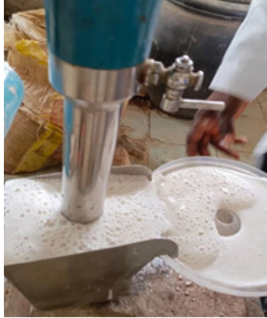
Figure 2: Froth floatation collection process
