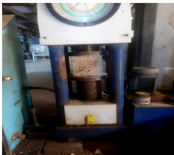
Figure 2: Compressive strength test setup for concrete cubes
