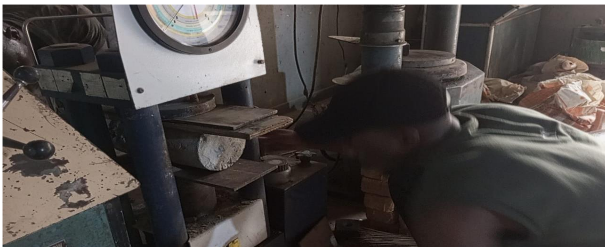
Figure 3: Split tensile strength test setup for concrete cylinders
