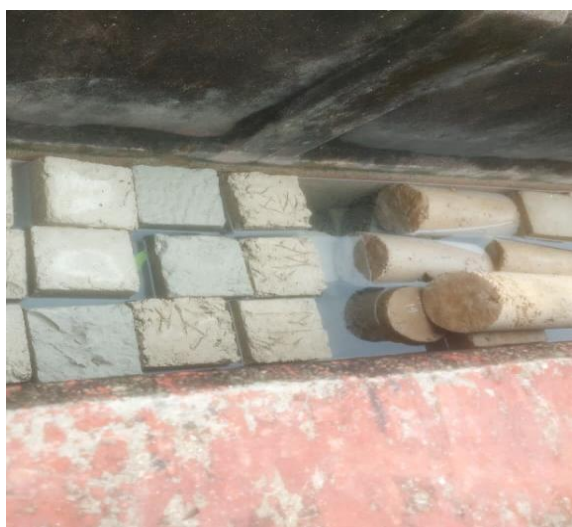
Figure 1: Curing of concrete cubes prior to mechanical testing
