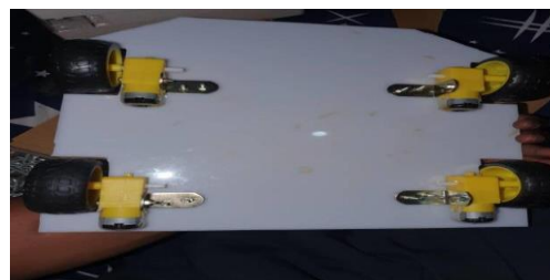
Figure 4: Attachment of DC motor and wheels
