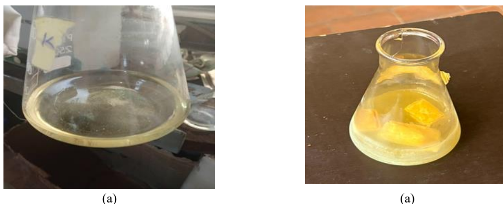
Figure 3: (a) Beginning of extract formation in solution due to decomposition (b) Decomposition of the composite in 6M Nitric acid after 14 days
